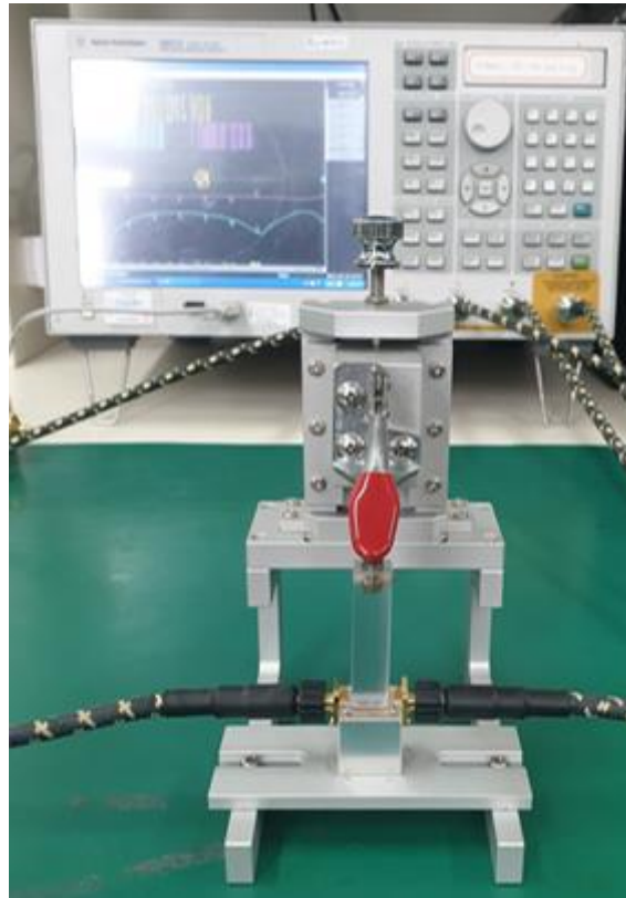
Figure 5. Test Setting to Measure the ATS1020N30 S-parameters
