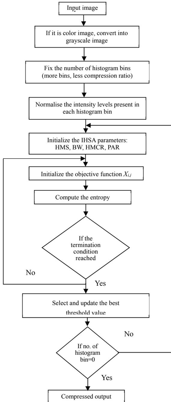
Fig. 1. Working model of OIHS based image compression.
