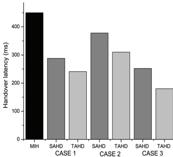
Fig. 20. Handover latency observed in each VHO method.
