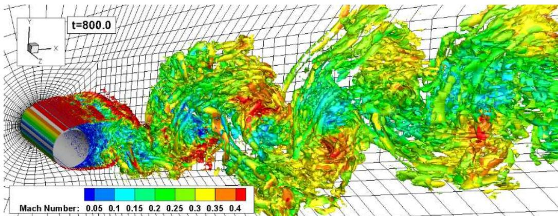
Figure 1. LES analysis of a transitional flow over a circular cylinder.
