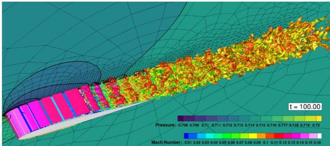
Figure 2. LES analysis of a transitional flow over the SD7003 airfoil.
