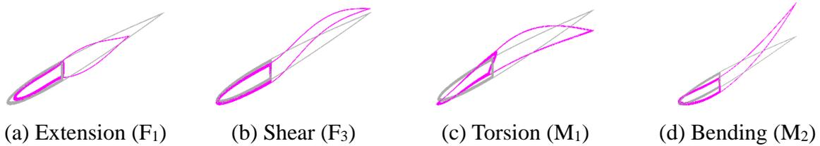
Figure 2. Selected warping deformations of blade
