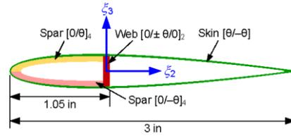
Figure 1. Schematic of composite blade
