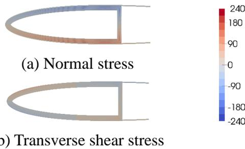
Figure 3. Reactive stress coefficients of blade
