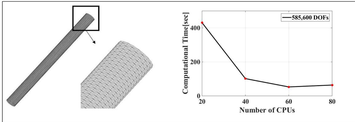
Figure 1. Three-dimensional configuration of structures and the decreasing trend of computational time
