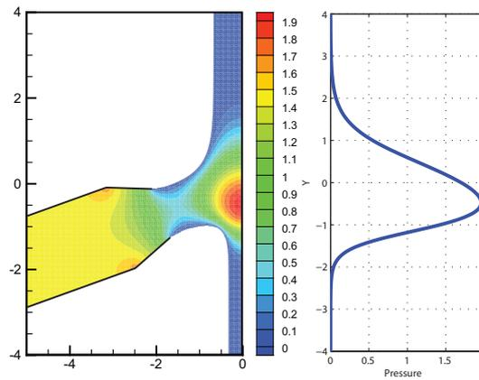
Figure 1. Isobaric plot of the excess pressure of the jet flow in case of the angled nozzle.
