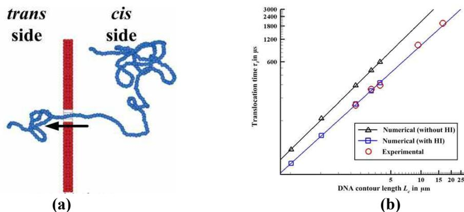
Figure 1. (a) Configuration of a polymer chain in the middle of the translocation process (arrow indicates translocation direction), and (b) variation of translocation time with polymer length.
