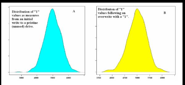
**Fig. 5.** This example displays the experimentally derived magnetic field density functions for hard drive rewrites where "A" displays the measured distribution of binary "1" values on initial copy. "B" displays the distribution of values associated with a binary "1" value following an overwrite with another binary "1".
