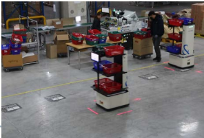
AGABANG Logistics Center Lightweight Rack, B2C, High-Mix, Low-Volume, Multi-Order Picking
